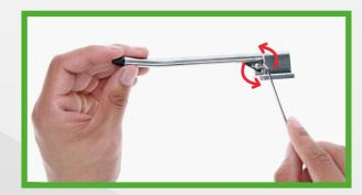
**3.** Place the new blade on the air nozzle and turn the bolt clockwise until it is secure. Note: Hand tighten only. Over tightening can cause the blade to break.
