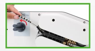
**2.** Holding the tip of the air nozzle, use the provided tool to turn the bolt counterclockwise to remove the blade.
