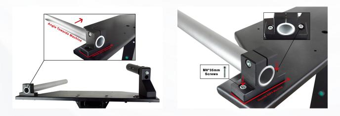
**Step 4:**Using the two M8\*35mm screws, secure the film leading bar module to the installation table. **Note:**Adjust the bar to be angled 3cm towards the machine, reference picture for details.
