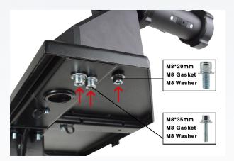
**Step 3:**Secure the roller module to the installation table using two M8\*35mm screws and one M8\*20mm screw, reference the picture for correct screw placement. All screws will use M8\* gaskets and washers.
