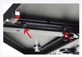
**Step 7:**Secure the sensor to the installation table using M3\*12mm screw and nut. Sensor wire will be secured using the rubber clamps under the installation table.
