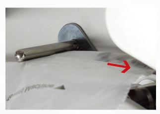
**Step 12:** On the side of the film that is closest to the machine, create a small opening and thread film through the feeding tube up to the belts.
