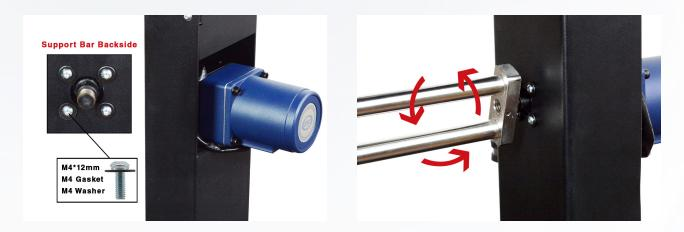
**Step 5:** Install the winder motor to the support bar using four M4\*12mm screws, gaskets, and washers. Attach the winder rods to motor by rotating counterclockwise. Turn until hand tight.
