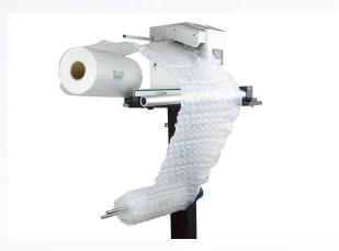
**Step 17:** Machine should be creating air pillows and winder should be spinning.
