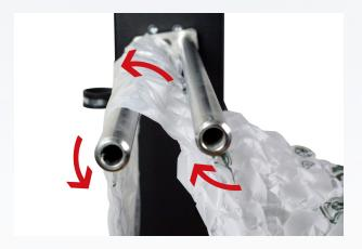
**Step 15:** Hit stop. Once stopped, align the film to go in-between the fork rods.
