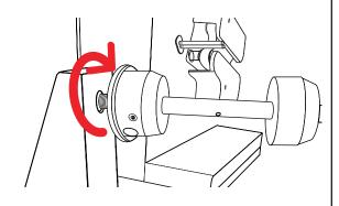
4. SCREW FILM ROLLER INTO FILM HOLDER AND HAND TIGHTEN.
