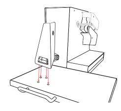
3. PLACE PLATFORM UPRIGHT. LINE UP FILM HOLDER WITH THE 4 SCREW HOLES AND SCREW IN WITH INCLUDED WASHERS.
