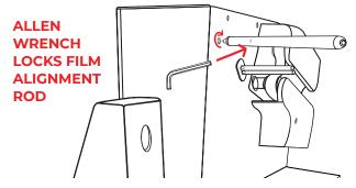
5. INSERT THE FILM ALIGNMENT ROD (LOCATED IN THE FOAM PIECE) INTO THE MACHINE AND THEN INSERT ANY OF THE INCLUDED ALLEN WRENCHES INTO THE HOLE INDICATED ON THE IMAGE ABOVE. USE THE ALLEN WRENCH TO HELP TURN THE ROD CLOCKWISE AND SECURE THE ALIGNMENT ROD TO THE MACHINE. REMOVE ALLEN WRENCH ONCE SECURED.
