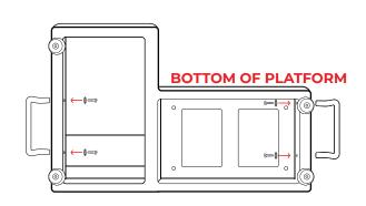
1. **INSTALL THE HANDLES ON BOTH SIDES** OF THE PLATFORM USING THE APPROPRIATE ALLEN WRENCH AND SCREWS WITH WASHERS.
